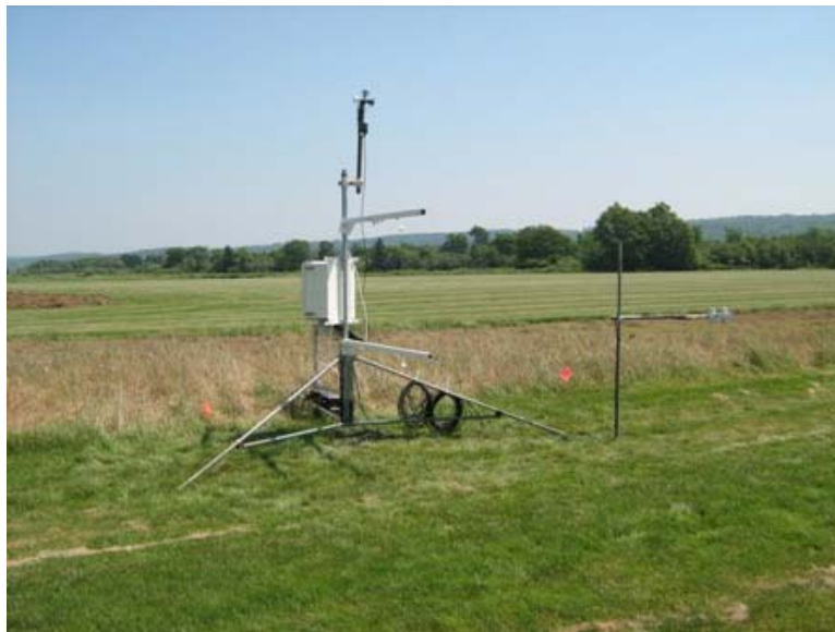
Fig. 1. Set up of CSI Bowen Ratio equipment on East of field.
